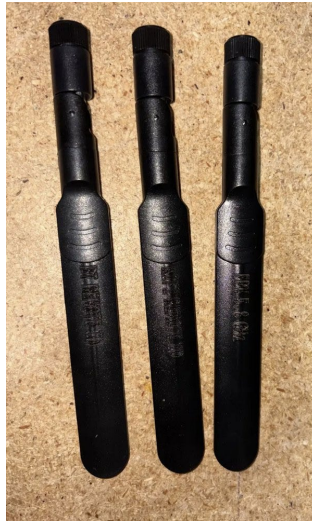
Figure 9 — The three dual-band antennas. Read the etched label at the base of each before installing.
