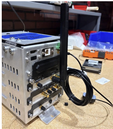
Figure 6 — DRAGON SDR antenna installed
