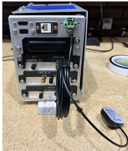
Figure 4 — GPS antenna installed below the DC terminal block, cable routed clear of the panel
