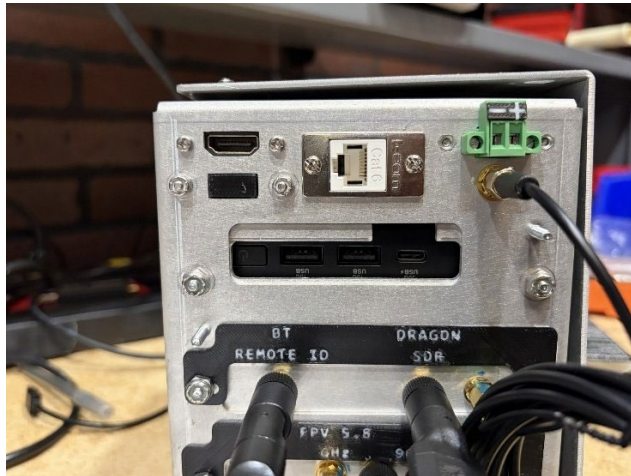
Figure 12 — Dust cover removed on an Elite Drop-In, exposing the compute power button and USB ports
