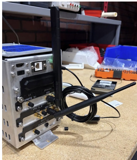
Figure 8 — 900 MHz antenna installed
