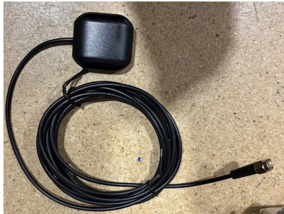
Figure 3 — GPS puck antenna with integral cable and SMA male connector
