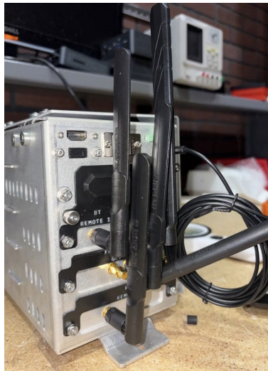
Figure 10 — Dual-band antennas installed
